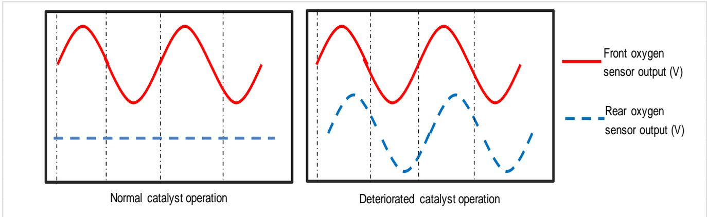
Figure 5: Variation of front and rear oxygen sensors
