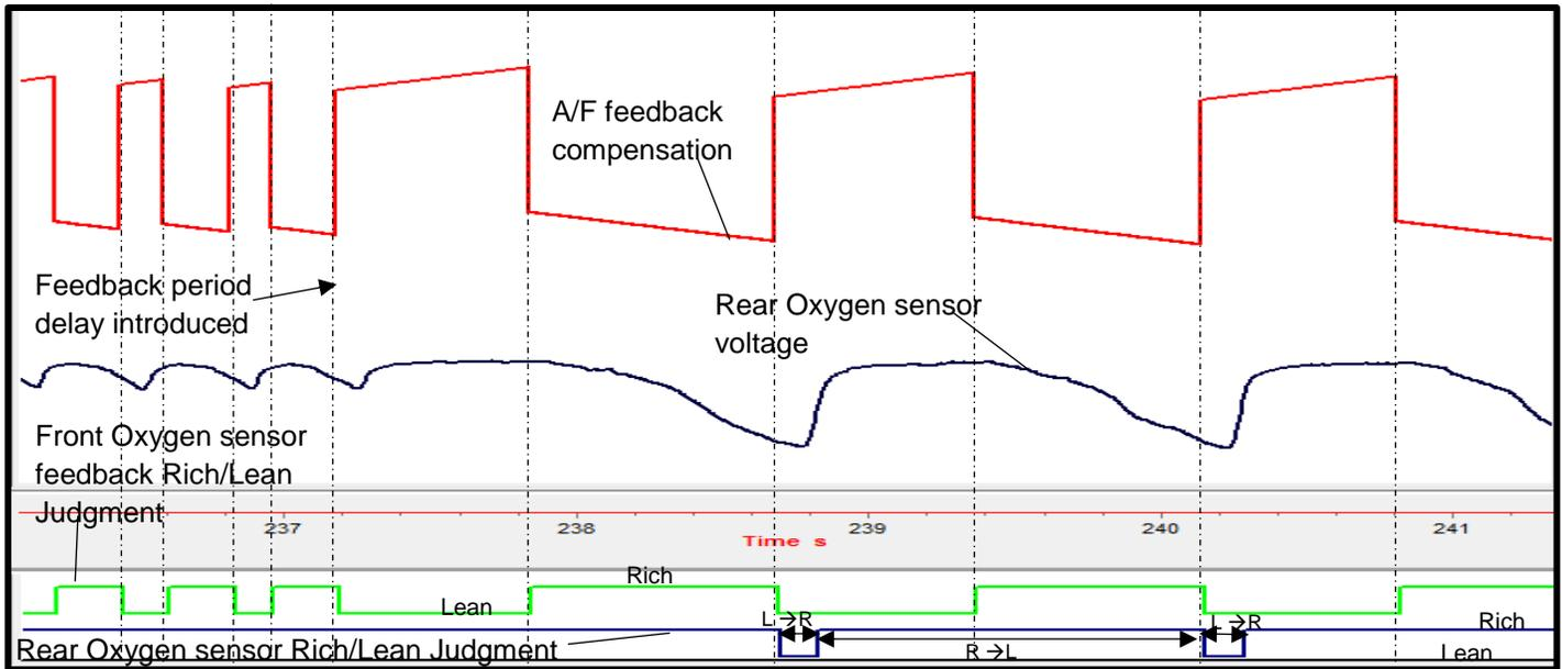
Figure 7: Introduction of feedback delay for catalyst monitoring
