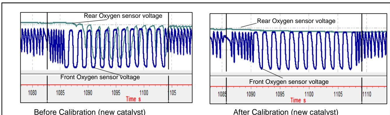
Figure 10: No fluctuations in rear oxygen sensor voltage after re-calibration in CNG mode
