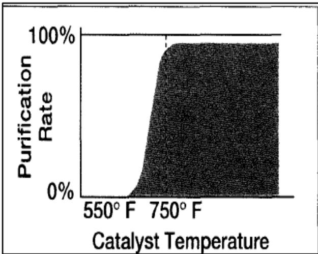
Figure 2: Catalyst efficiency variation with temperature
