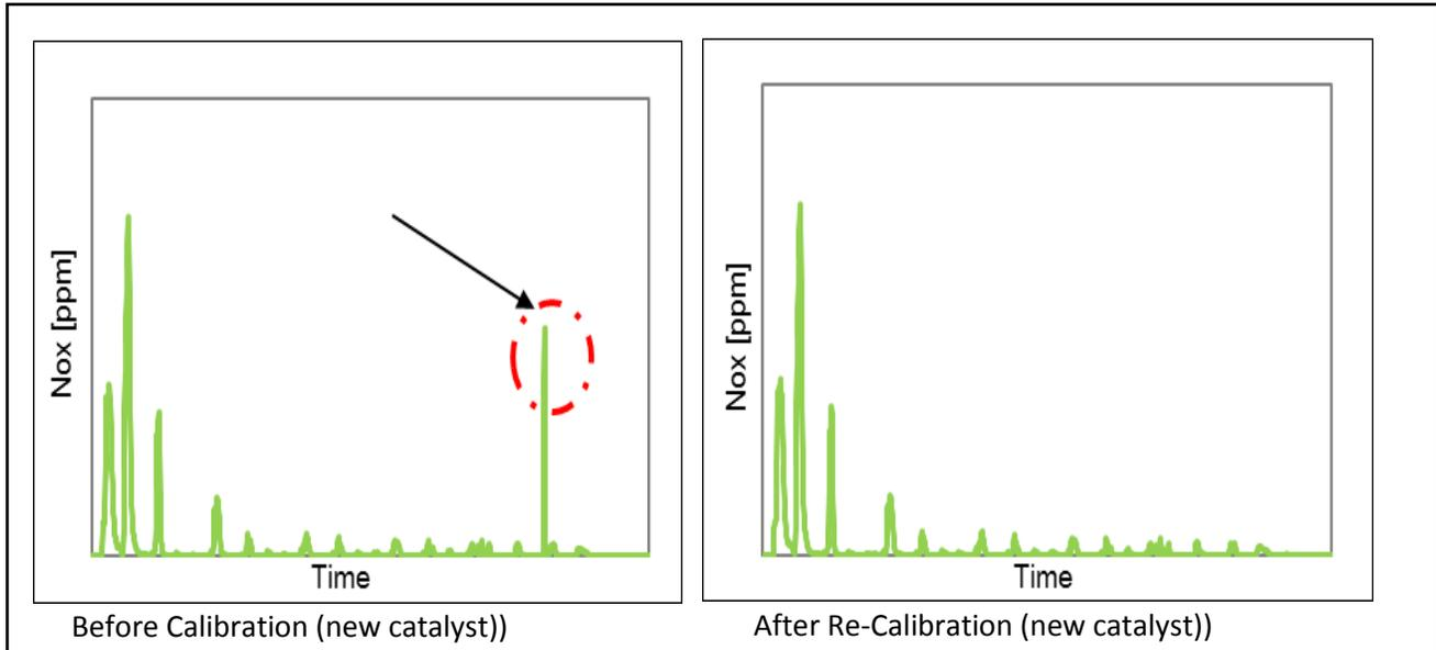
Figure 11: NOx peak during catalyst monitoring
