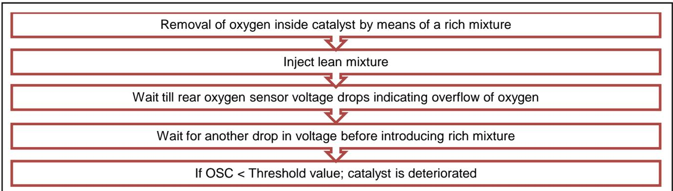
Figure 6: Catalyst Monitoring using active method
