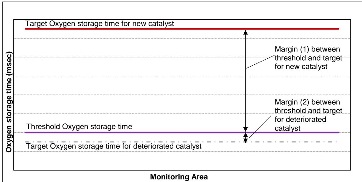
Figure 9: Oxygen storage time margins setting for deteriorated and new catalyst
