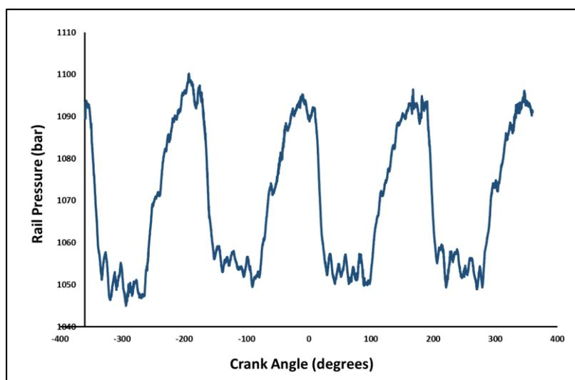
**Fig.8 Variation of Rail Pressure in one cycle in mHawk Engine**
