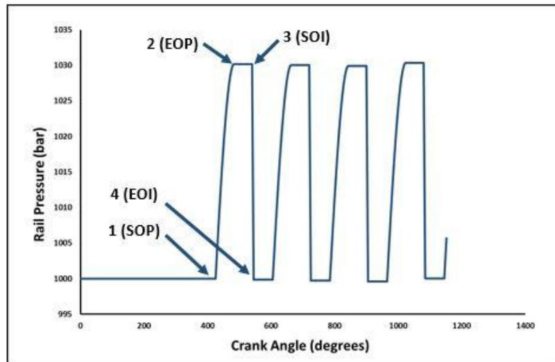
**Fig.7 Variation of rail pressure in one engine cycle**
