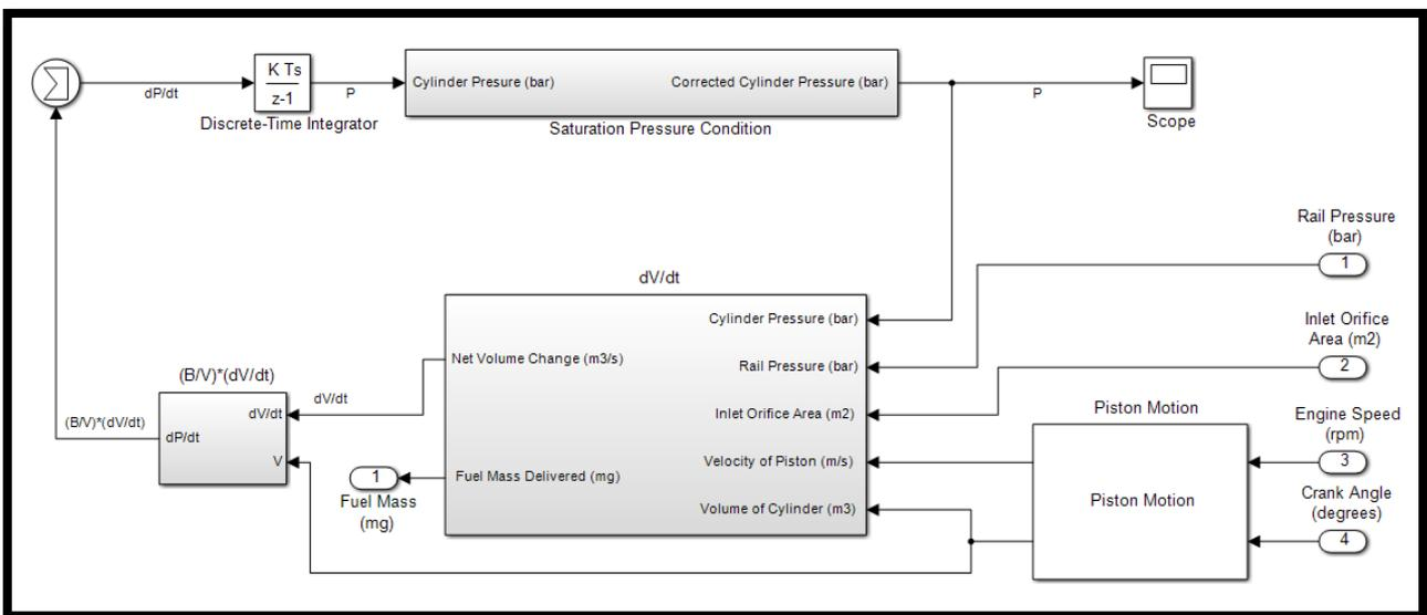
Fig.3 Simulink model of high-pressure pump (one cylinder)
