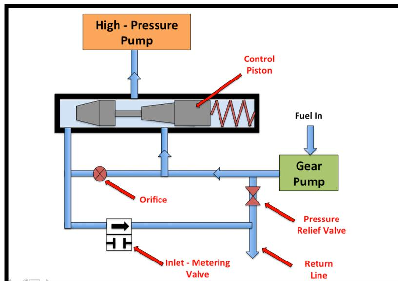
Fig.1 Schematic of the common rail pump with IMV
