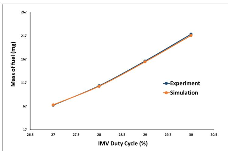
Fig.6 Comparison of mass of fuel delivered by pump in 1 cycle
