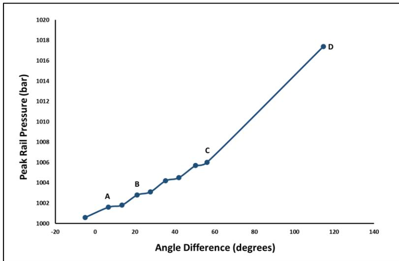
Fig.9 Variation of Average Rail Pressure with Injection Timing
