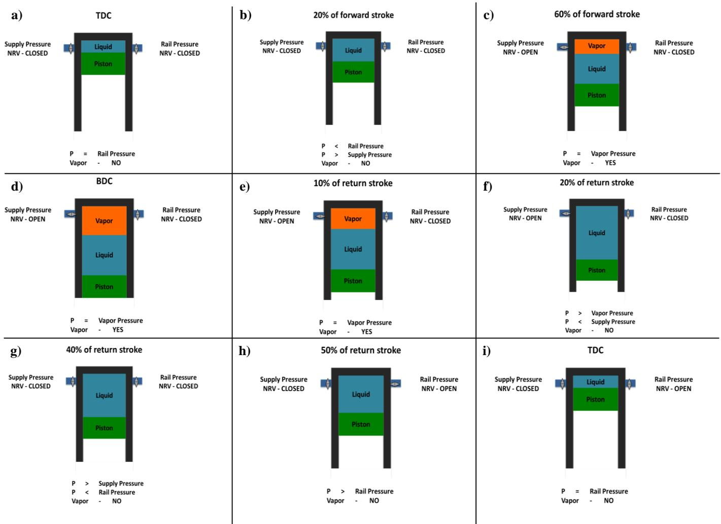
Fig.2 Stages of vapor formation inside the cylinder in one pump revolution
