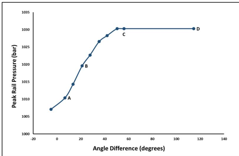
Fig.10 Variation of Peak Rail Pressure with Injection Timing
