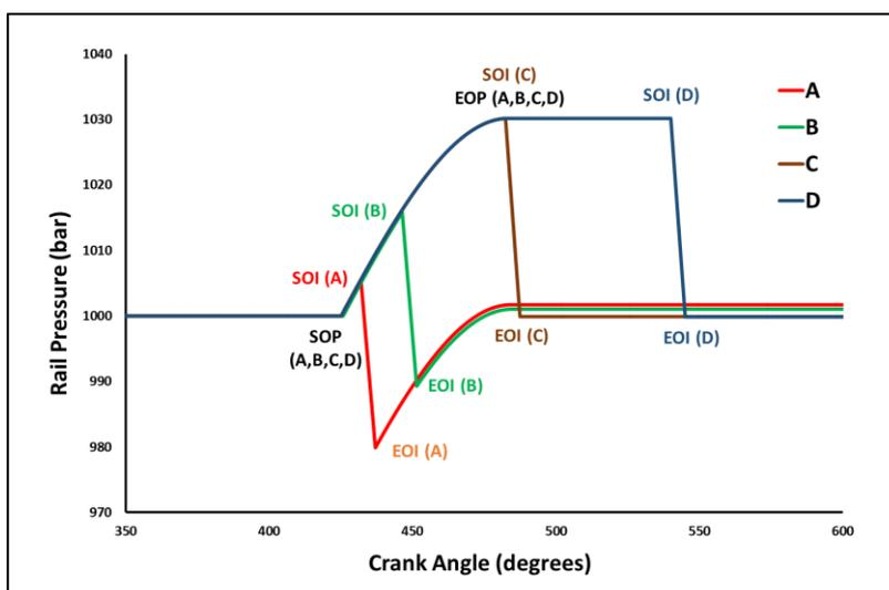
Fig.12 Variation of Rail Pressure (one fourth cycle) for 4 Injection Timings
