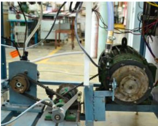
Fig.4 Motor and Angle Encoder
