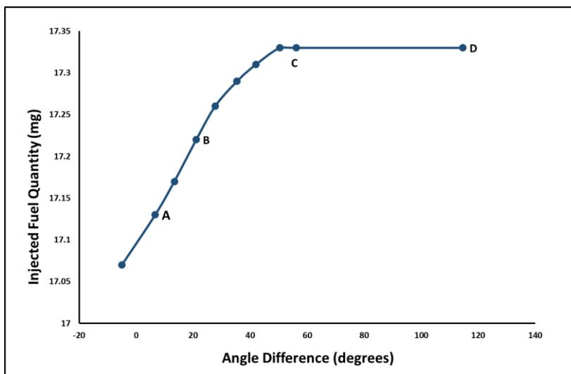
Fig.10 Variation of Fuel Quantity Injected with Injection Timing
