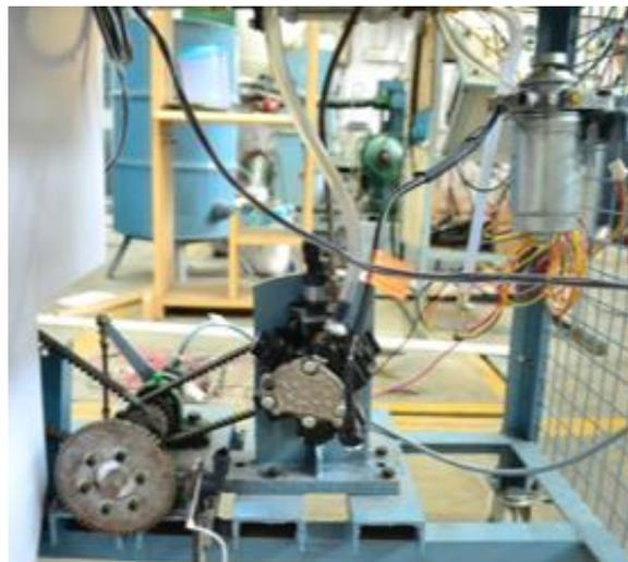
Fig.5 High-Pressure Pump and Trigger Wheel
